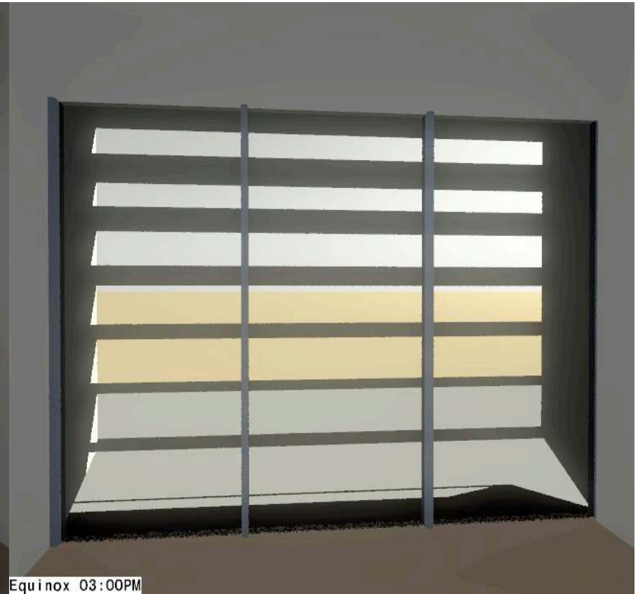
View with Recommended Sunshade Modification
